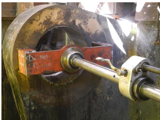
Boom foot lug upgrade and line boring
