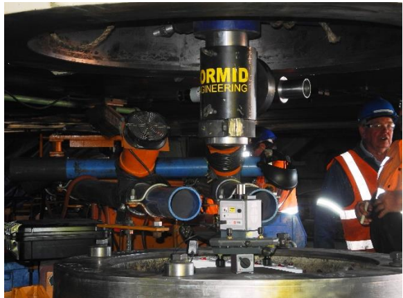
Laser alignment during rack and rail pad machining
