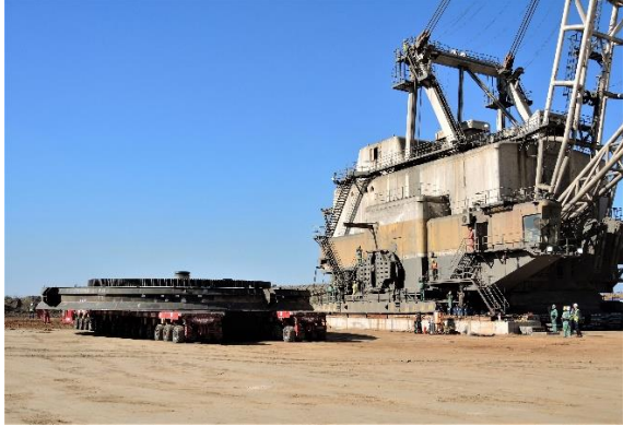
1570w tub relocated in one piece from one site to another
