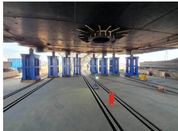
8 x 400 Ton and 6 x 250 Ton jacking system to lift entire dragline while on "high cam" and tub removed to refurbish the propel mechanisms
