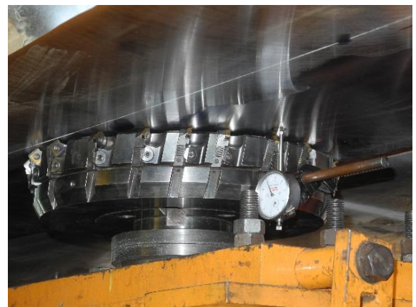
Machining of slew bearing lower and upper rail support pads with self-leveling machining
