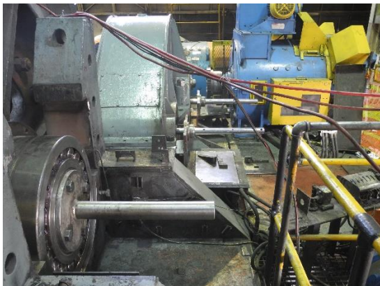
Hoist and drag gear cases alignment check and insitu line boring
