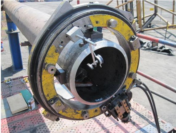
Insitu machining of boom chord and lacing weld preparations during chord replacements
