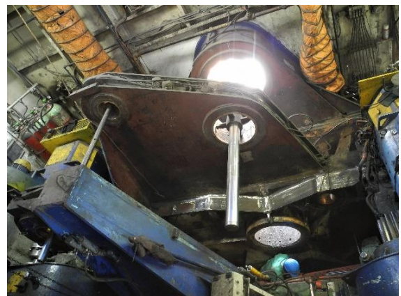
Propel girder hub alignment check, stock-welding and line boring
