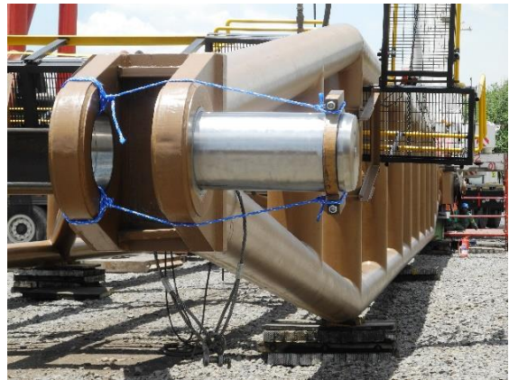
Boom and mast foot clevis upgrade and line boring
