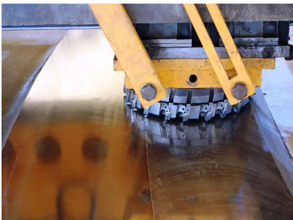
Machining of slew bearing lower and upper rail support pads with self-leveling machining
