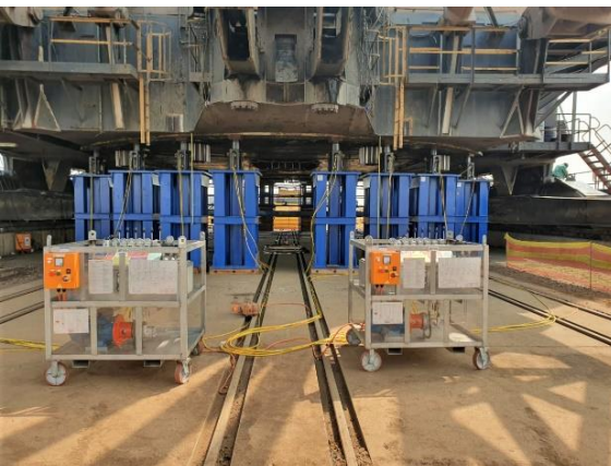
8 x 400 Ton and 6 x 250 Ton jacking system to lift entire dragline while on "high cam" and tub removed to refurbish the propel mechanisms
