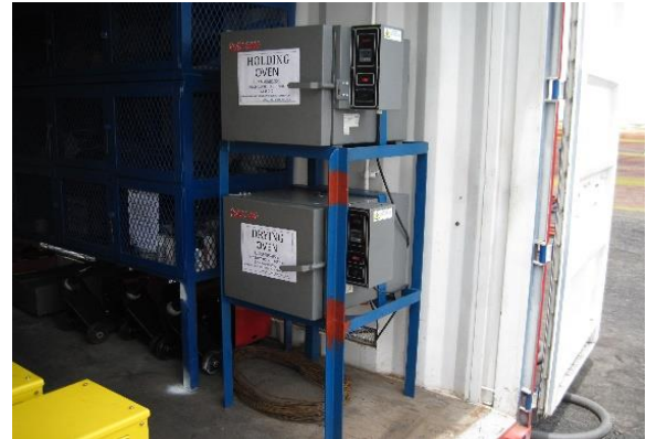
Electrode baking and holding ovens with appropriate electrode management system
