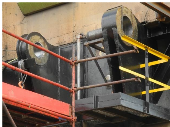
Boom foot lug upgrade and line boring
