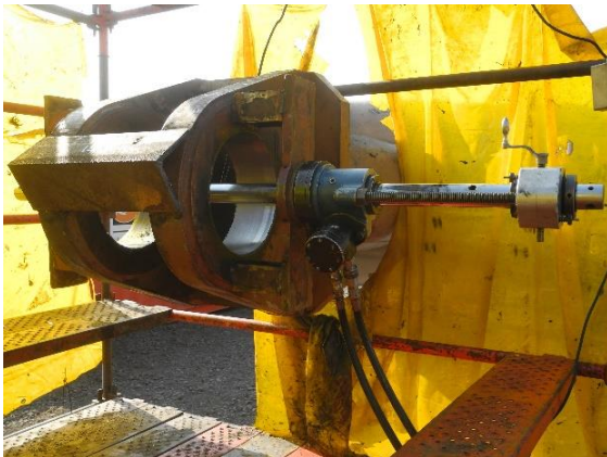
Boom and mast foot clevis upgrade and line boring
