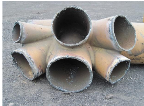
Boom refurbishment - Major chord upgrade and replacement
