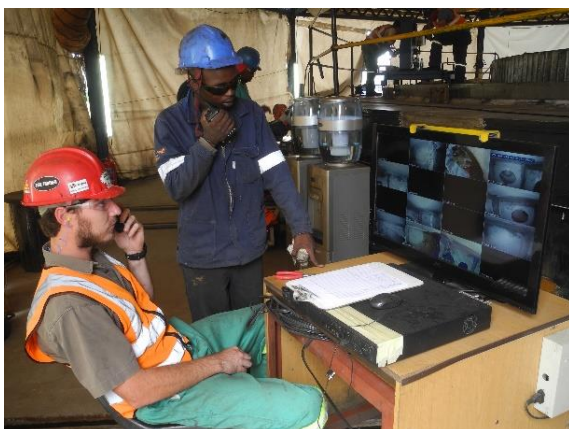
Confined space camera monitoring system and spotters
