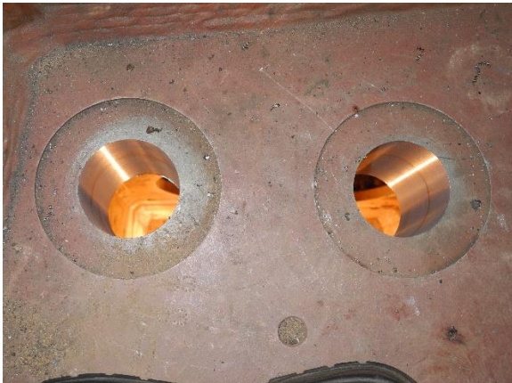
Rack segment mounting bolt holes drilled and reamed
