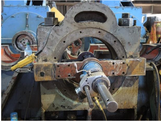
Hoist and drag gear cases alignment check and line boring
