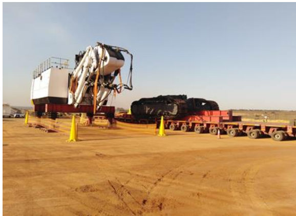
CAT 6060 Shovel tear-down, relocation and rebuild
