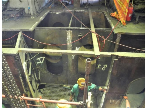
Marion 8200m major revolving frame refurbishment
