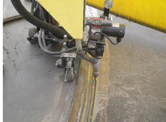
Sub-arc welding process provides the best quality and significantly save cost and time
